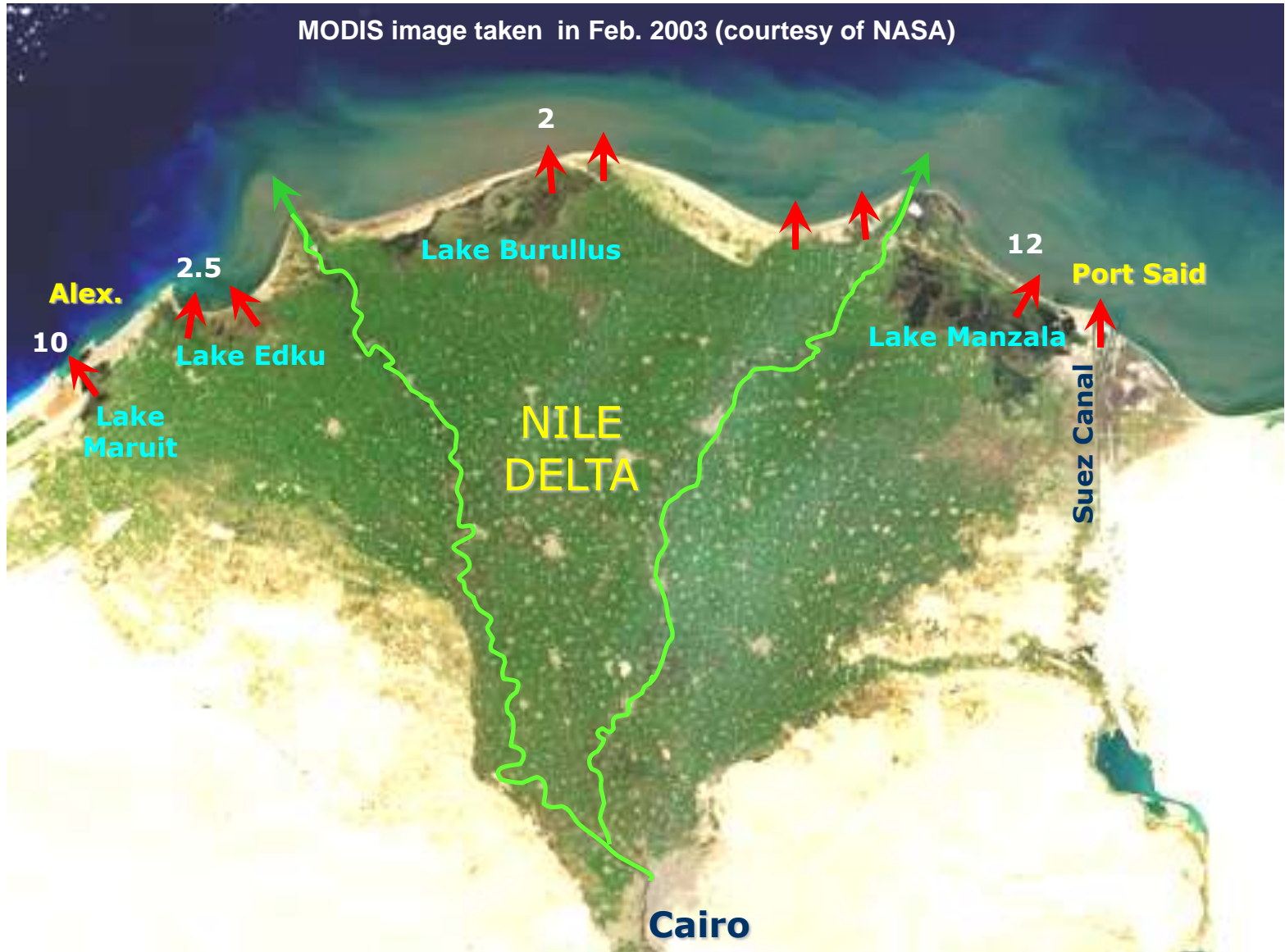
Major outfalls / land-based sources along the delta coast and quantities of effluents discharged each day (in million m 3 )
